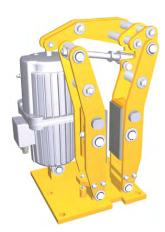
**MATERIAL:** construction of the brake – steel; brake shoes – spheroidal iron cast; asbestos--free friction lining; ZE thrustor body – aluminium, ExZE – iron cast; bolts made of stainless steel, self-lubricating sleeves.
